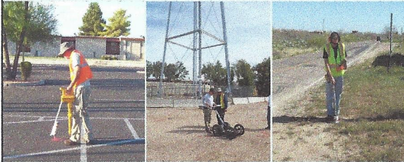
Electromagnetic Ground Penetrating Radar Acoustic
